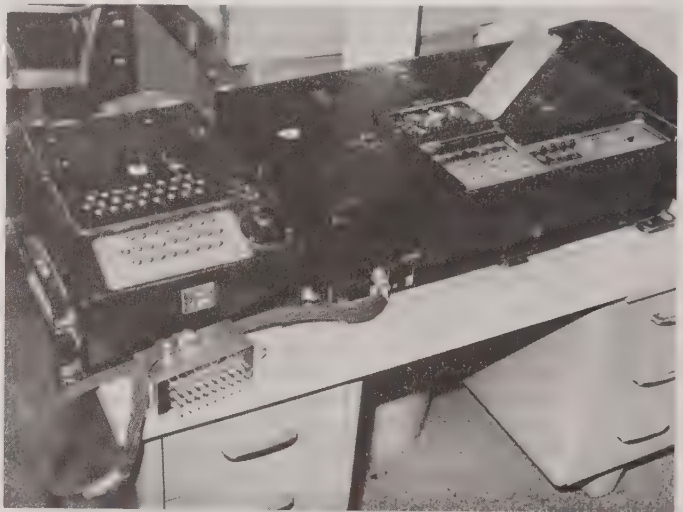
Figure 13: Japanese JADE cipher machine, a member of the PURPLE family of cipher machines.
